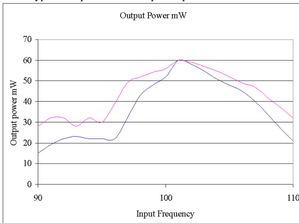
The upper curve is optimised output using snowflake tabs to the stubs. The lower curve is output from the PCB without snowflake tabs. The trimmers may be re-tweaked but its advisable to do this with minimum input drive. CV1 will only tune correctly with small input signal level this is due to the damping effect of D2 to provide drive level control.
